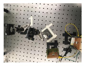
Figure: Collimating Light Beam with 2 Plano-Convex Lenses
