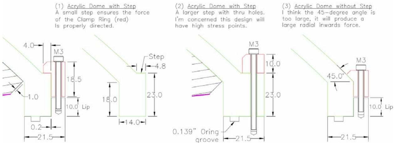
**Figure 1** This shows; (1) The proposed Oring face-seal for the Acrylic Dome (green). The dome has a small 4.8mm step so the force from the Aluminum clamp ring (red) is properly directed. (2) shows a design with a larger step and thru holes. I'm concerned this design would have high stress points at the screws. (3) For a Dome without a step, half the force from the clamp ring would be directed inwards. I don't like this and it may not work properly.
