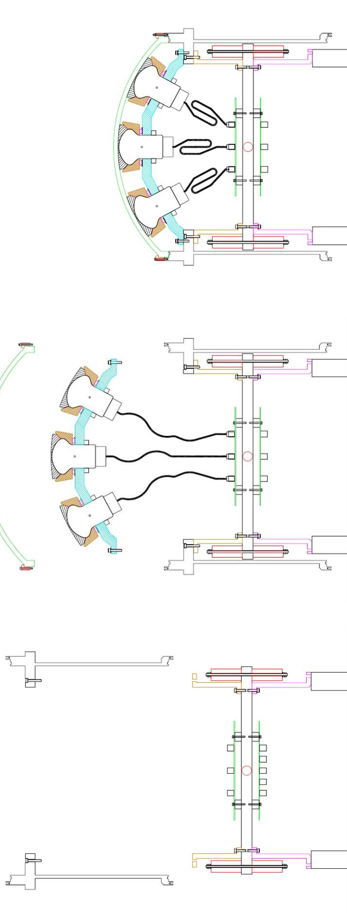
(1) Assemble Internal Components – Central Plate, RO Electronics, Ballast, two types of Support Brackets. Mount on Temporary stand. Install Cover. Connect Cover output Cables to the RO Electronics.
