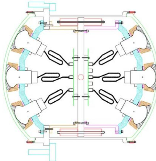
(6) Top View (top) and Section View (bottom) thru the support brackets. This shows the support brackets holding the nuPRISM Inward-Facing PMTs, and the brackets. The support brackets connecting the central plate to the six cover "tabs" also provide the conduction cooling of the electronics to the water.
