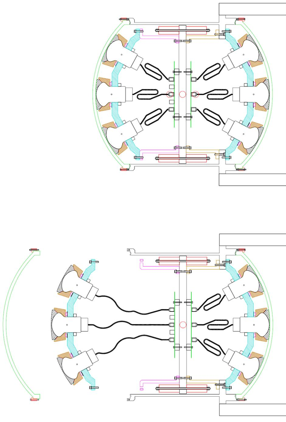
(4) Rotate assembly 180 degrees and mount on a second Temporary stand. Position Printed 19-PMT Support (with PMTs) ~150mm above assembly, reach in and plug PMT cables into Internal Electronics.
