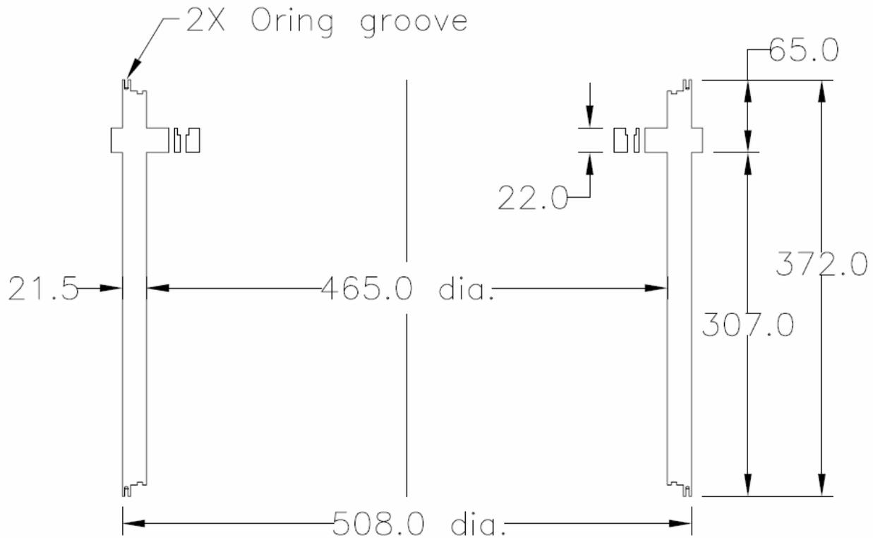
**Figure 6** This shows the same Cover with straight cylindrical wall.
