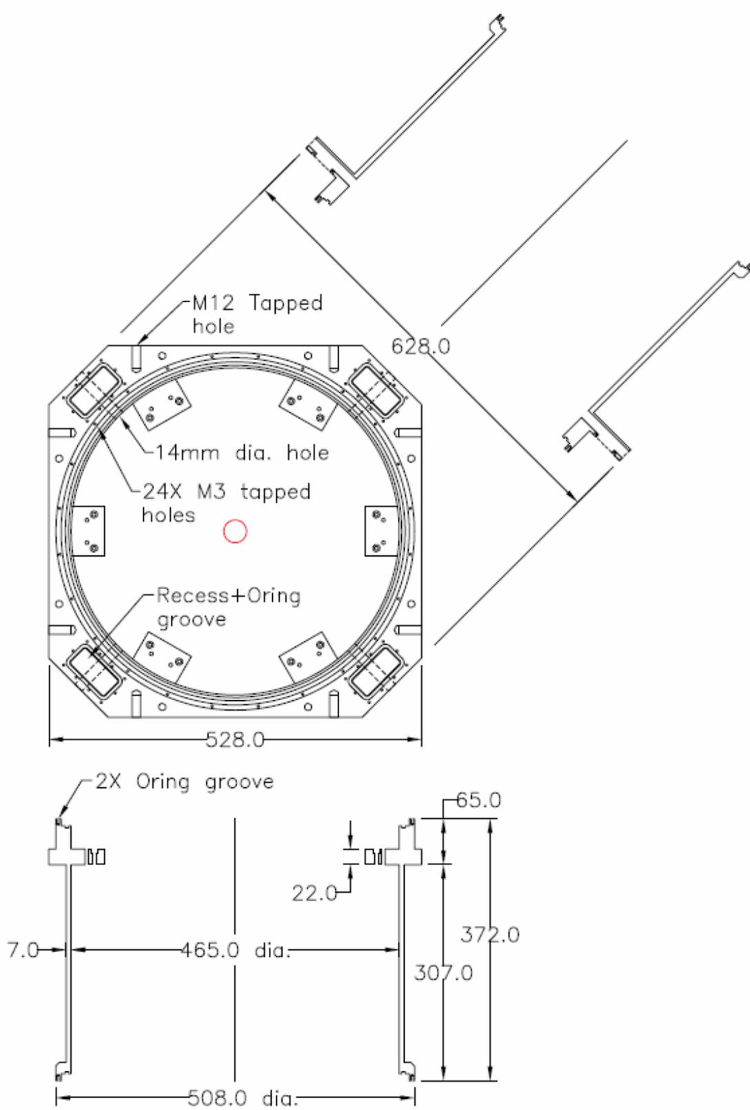
Figure 5 This shows the complex Cover required to eliminate two Orings.
