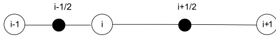
Fig. 1. The adopted nomenclature for finite differences. Mesh nodes are numbered by the integer index i (white circles). Discretization of the continuity equation (2) requires approximation of the current at mid-points of the mesh line connecting neighboring nodes (black circles).
