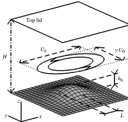
FIGURE 1. Three-dimensional set-up: a rotary barotropic tide of velocity amplitude  $U_0$  along its major axis and  $\gamma U_0$  along its minor axis flows over a topography of height  $h_0$  and typical slope  $h_0/L$ . The buoyancy frequency  $N$  and the Coriolis frequency  $f$ , both constant, are not represented. Note that the width of the barotropic tidal ellipse does not scale with the width of the topography.
